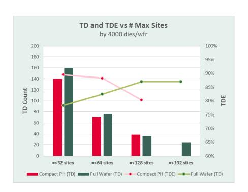
Full wafer contactors enables best TDE with highest parallelism
