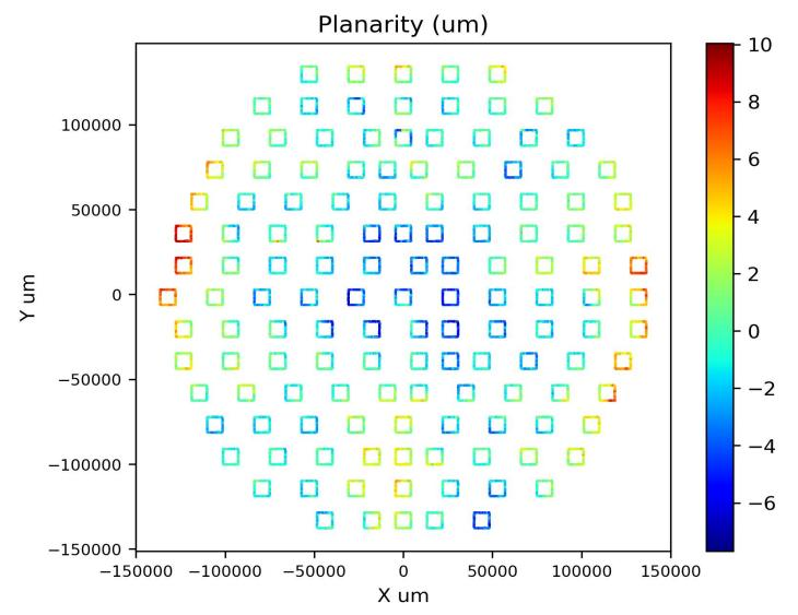
TSM provides excellent planarity of <20um across the full 300mm array
